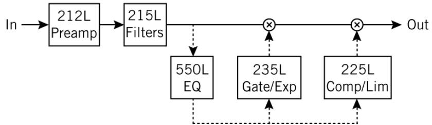
Figure 12. Signal flow with 550L SC enabled
