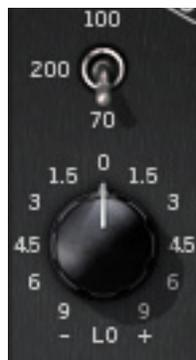
The low frequency (“LO”) shelf EQ has a selectable cutoff frequency which can be cut or boosted by various amounts.
