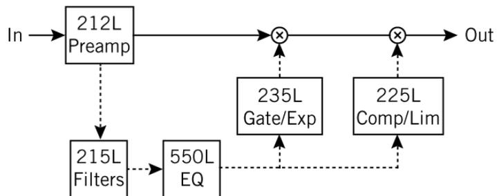
Figure 13. Signal flow with SC enabled in both 215L and 550L modules
