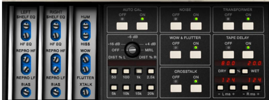
Figure 4. UAD Ampex ATR-102 secondary controls
