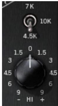
The high frequency (“HI”) shelf EQ has a selectable cutoff frequency which can be cut or boosted by various amounts.
